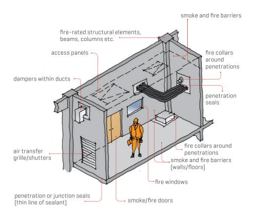
Figure 1. Passive fire protection building components
