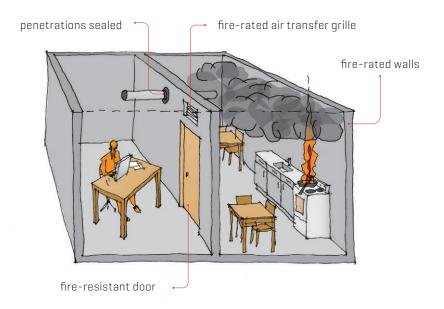
Figure 2. Fire spread control using passive fire protection
