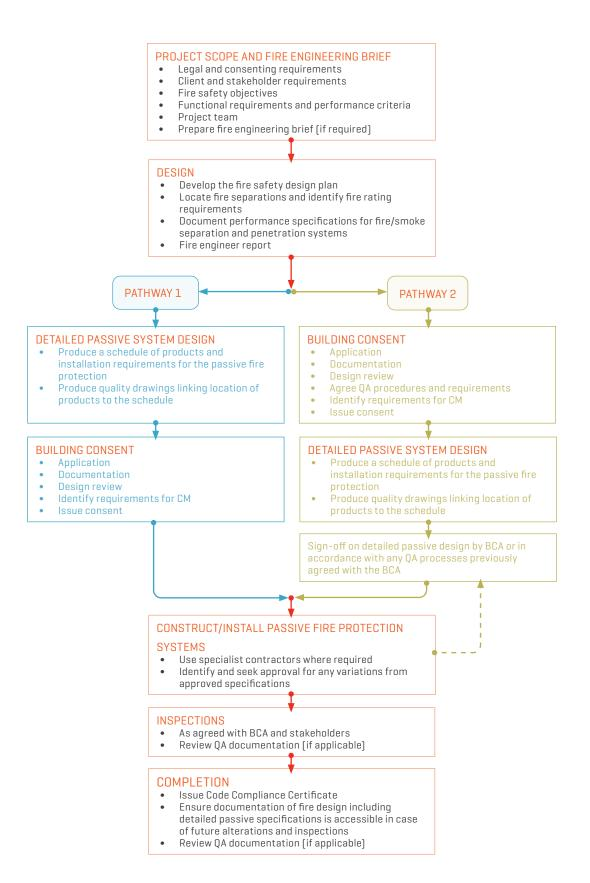
Figure 4. Typical project process for passive fire protection, showing two paths for specification and approval
