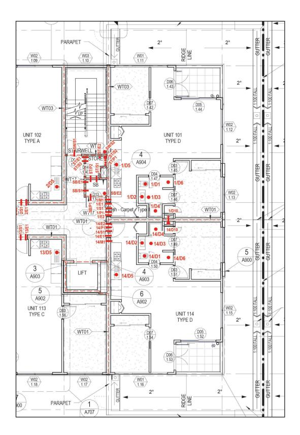
Figure 5. Example of plan of penetration seals
