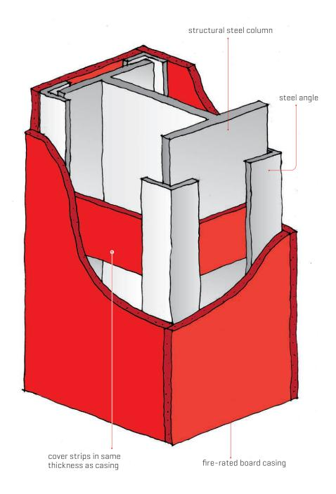
Figure 23. Structural fire protection – fire-rated boards protecting steel columns
