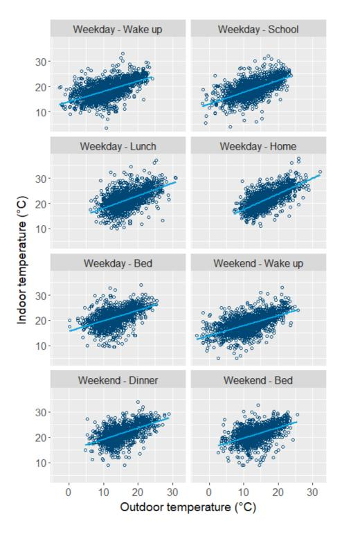
Figure 2. Correlation between Indoor temperature and outdoor temperature as recorded at the local NIWA weather station
